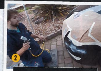
2 On goes the primer coat, covering the newly repaired surface
